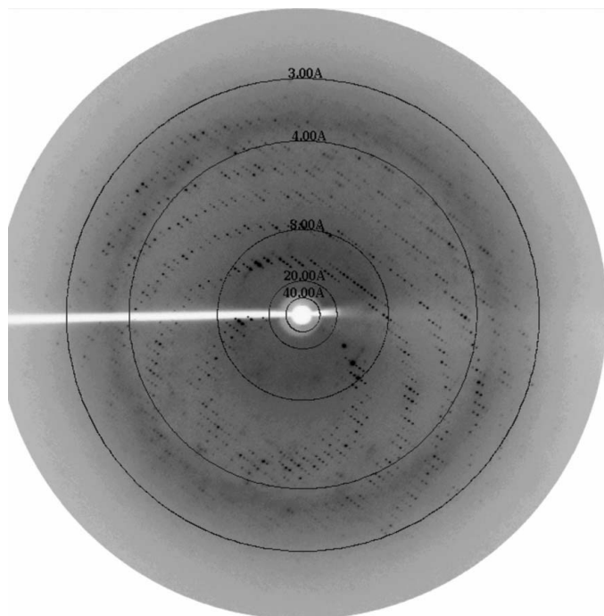
Figure 3 X-ray diffraction frame collected from a crystal of Sa239.
